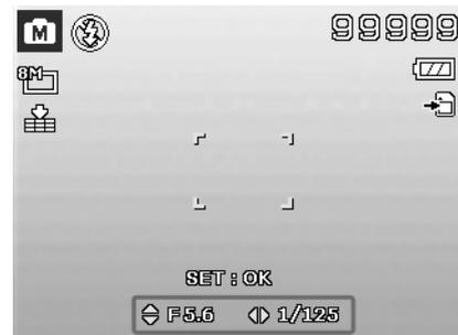
Displays the aperture and shutter speed value
